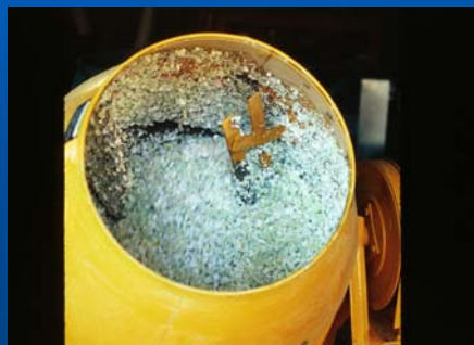
EPS, water, clay, and other components before mixing
